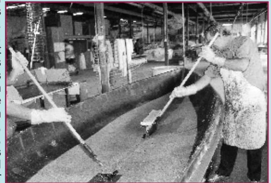
Resin-impregnated cloth is squeegeed to eliminate voids or bubbles
